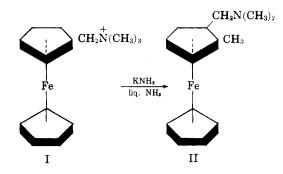
Quaternary ammonium ion I (as the iodide) gave, with potassium amide in liquid ammonia (two hours), a 60% yield of tertiary amine II, b.p.
